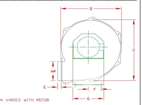
The Motor Frame is normally decided by the factory based on H.P. and the RPM of the fan. The 56 frame is normally used on up to 1 H.P. motors, and 143T is used up to 3 H.P. in most cases. If you require a specific frame for your selected motor, contact your dealer as some fans can interchange between motor frames for special needs.
