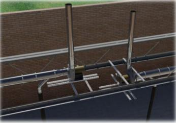
**Ceiling Joist Mounting-**Unistrut Hung from Ceiling Joists
