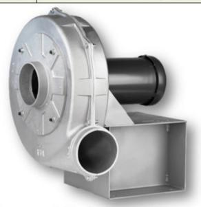
This exhaust fan is designed for the purpose of exhausting most particulates as well as volatile organic compounds (VOC's) created by internal combustion engines. These fans feature high pressure 3/16" minimum thickness radial flat wheels, direct drive, and are AMCA Type B spark resistant. Housing shall be of Aluminum/Magnesium alloy created by 2-piece construction with gaskets and steel hardware. Fan shall be tested and be in accordance with AMCA Standard 210.
